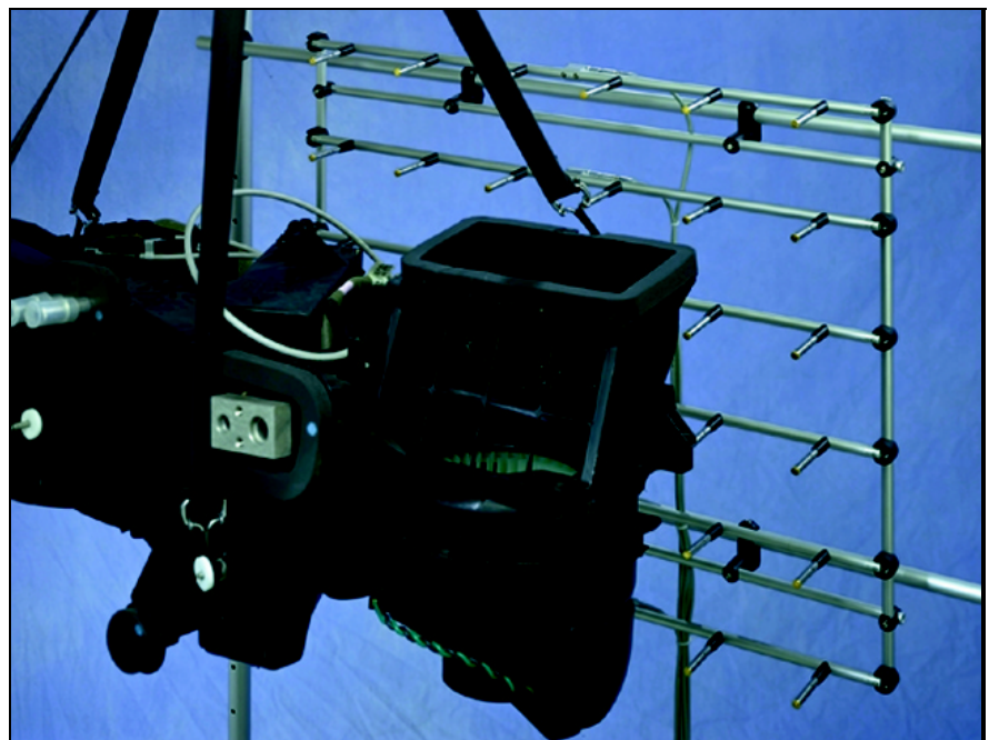
Fig. 1 Typical application of Array Microphone Type 4935. The noise pattern for a car fan unit is being analyzed using a microphone array and the Spatial Transformation of Sound Fields technique (STSF system Type 7688)
